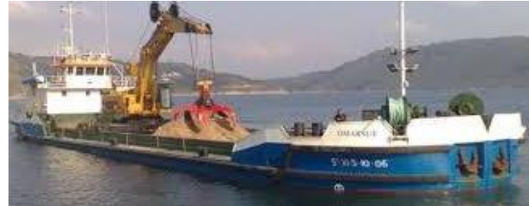
Illustration 17. SPLIT BARGE dredger
