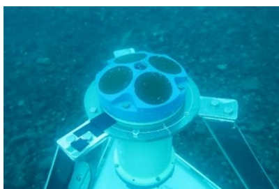
Illustration 99. ADCP moored in the Port of Las Palmas
